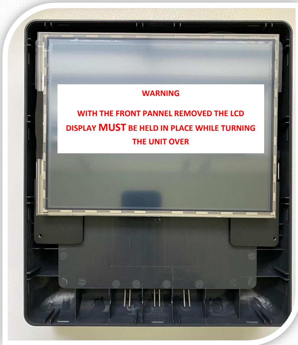
Figure 11 – Enclosure with Front Panel Removed
